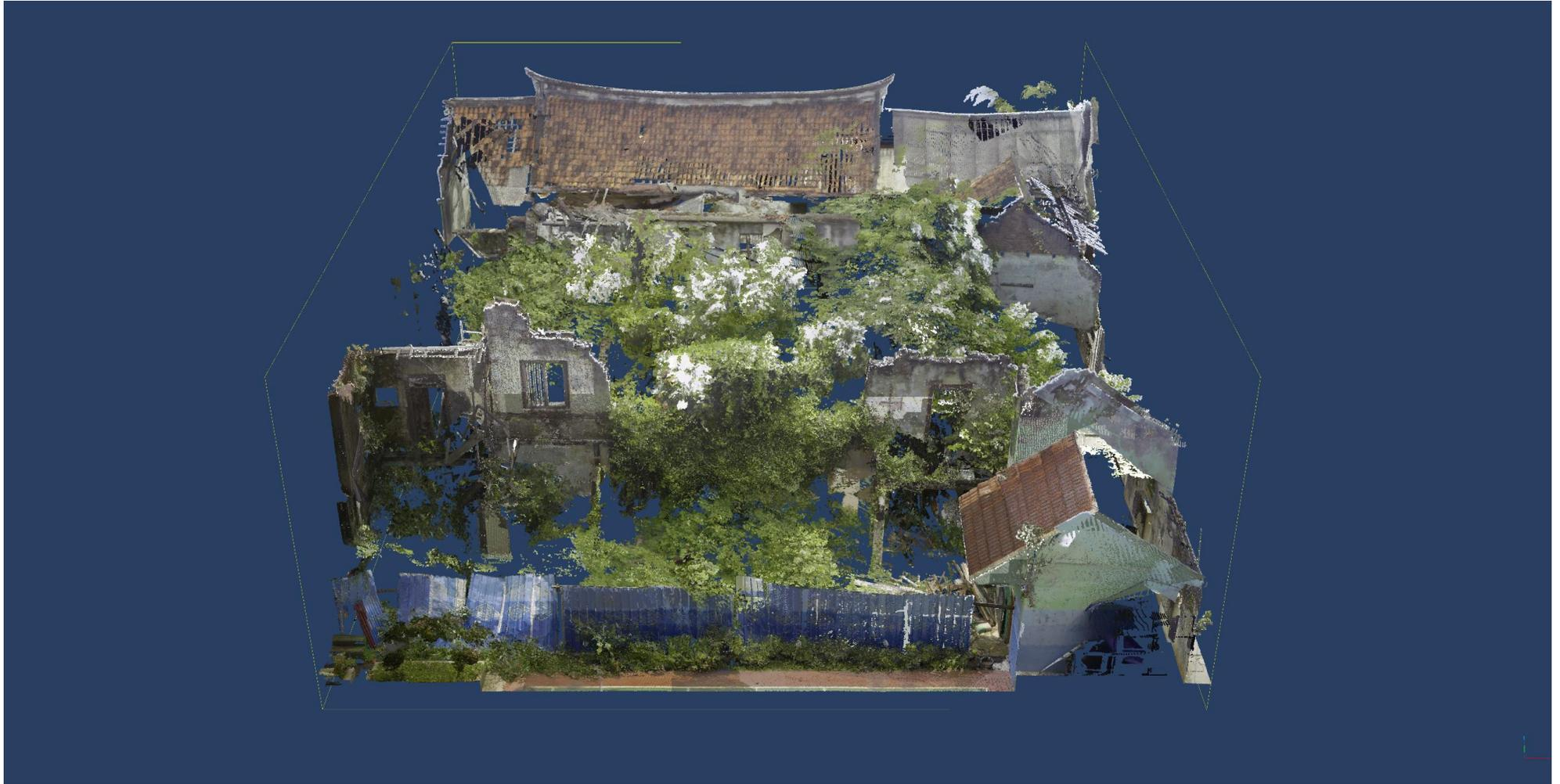
Gambar 17. Hasil pemindaian 3D laser scanning perspective view
