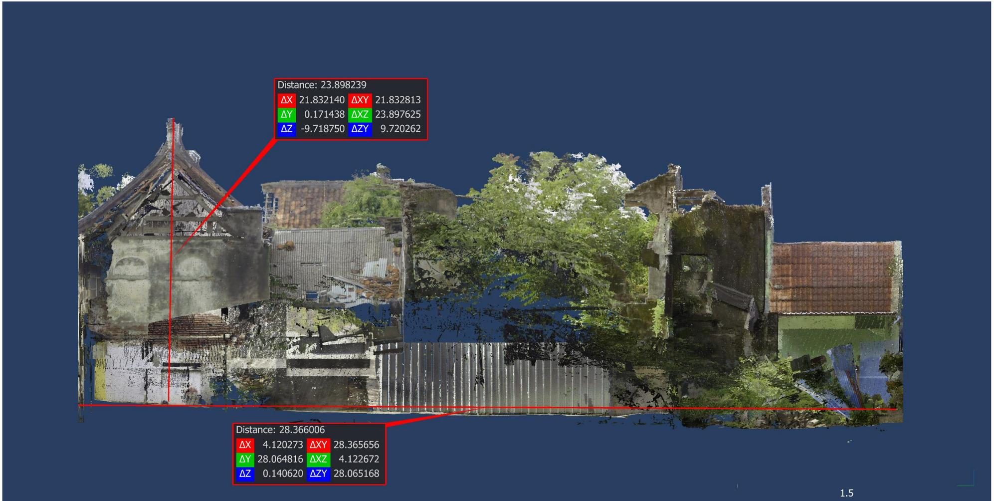
Gambar 20. Hasil pemindaian 3D laser scanning tampak samping kiri (left view)
