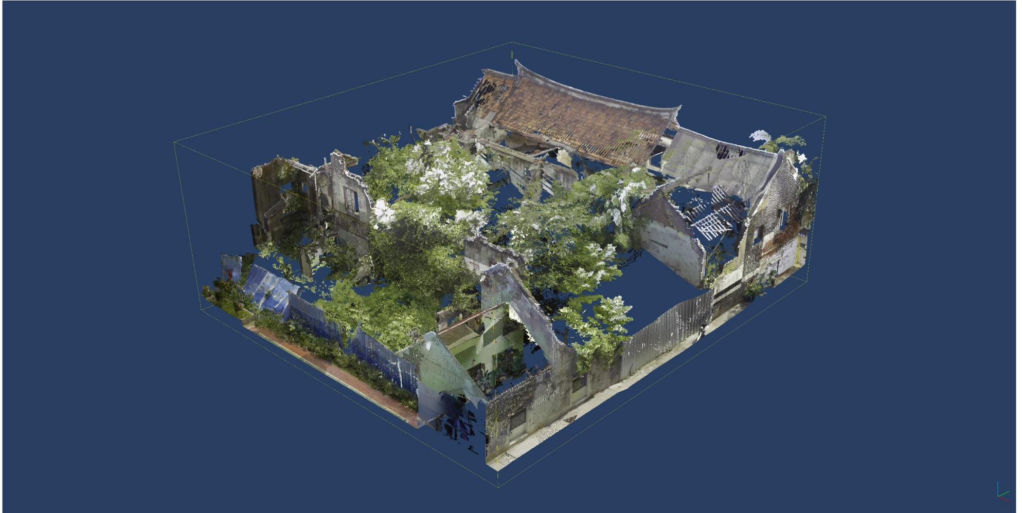
Gambar 16. Hasil pemindaian 3D laser scanning perspective view
